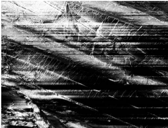
In this comparison of fibre glue sample the excellent benefit of the ULTRAplus charge compensator is demonstrated. Left: The sample charges up extremely at 5 kV primary energy with gas flow of charge compensation turned off. The image is disturbed by jittering and arcing. Right: With turned on charge compensator the fine details of the fibre glue surface are visible. Image is taken with chamber mounted Everhart-Thornley detector at 5 kV.
